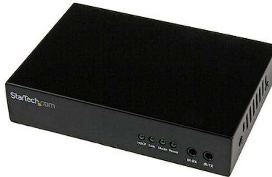
This HDBaseT receiver works with the ST424HDBT HDMI matrix switch to extend an HDMI audio/video source up to 230ft (70m) over Cat5e/6 cabling. One STHDBTRX receiver unit is required for each individual remote display.
