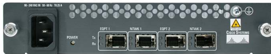
Figure 2. SFP Ports on the Transponder
